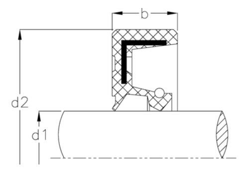
$\begin{array}{ll} b & = 8 \\ d1 & = 26 \\ d2 & = 42 \\ Material = NBR \end{array}$
